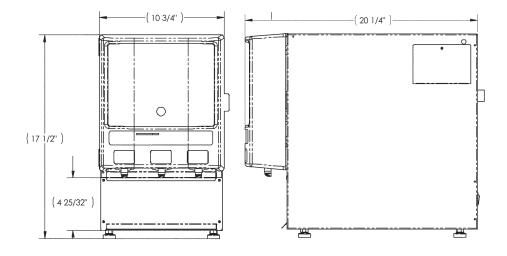
Specifications Shipping weight: 30 Lbs Body Construction: 300 series stainless Electrical:120 VAC 15 A Products: 3
